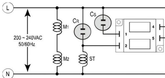
Cs: Start capacitor, Cr: Run capacitor, M1/M2: Main coil, ST: Auxiliary coil
