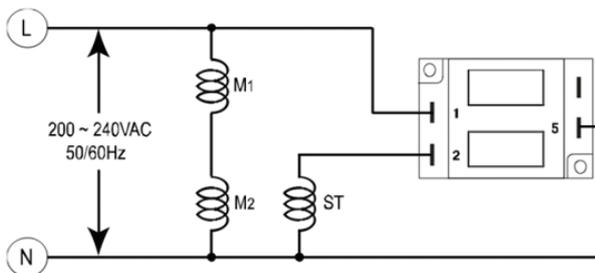
M1/M2: Main coil, ST: Auxiliary coil
