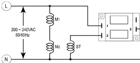
M1/M2: Main coil, ST: Auxiliary coil
