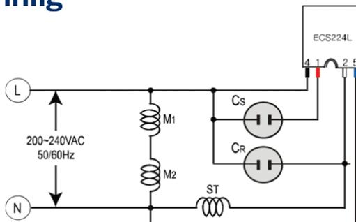
Cs: Start capacitor, Cr: Run capacitor, M1/M2: Main coil, ST: Auxiliary coil
